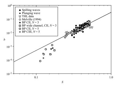
FIGURE 16. Plot of *b* versus *S* for SIO spilling and plunging waves along with the data of Melville (1994) and the THL data. Also shown are the data of Banner & Peirson (2007, BP). The solid line is a least-squares fit to the SIO data and has a slope of 2.77.
