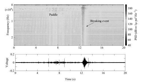
FIGURE 6. (a) Spectrogram and (b) voltage time-history of a hydrophone signal. The breaking event is seen as a broadbanded signal in the spectrogram.
