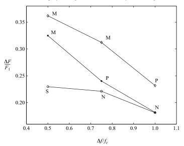
FIGURE 9. Normalized change in energy flux across the control volume as a function of bandwidth, with  $F_1$  the total energy entering the control volume. All packets have  $f_c = 1.08$  Hz and  $x_b k_c = 57.92$  with S = 0.32 ( $\circ$ ), S = 0.38 (\*), and S = 0.46 ( $\diamond$ ). The qualitative nature of the breaking is also noted, where N is non-breaking, S is spilling, P is plunging, and M is multiple breaking.
