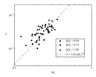
FIGURE 13. Plot of b versus the local slope,  $hk_c$ . Data for all three bandwidths for singly breaking plunging waves only are shown. The dashed line is a fit of the data to the curve  $b = \alpha (hk_c)^{5/2}$ , where  $\alpha = 1.03$ .
