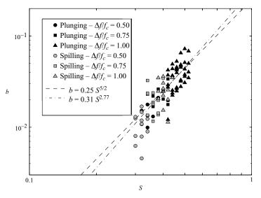
FIGURE 14. Plot of b versus the input slope, S for singly breaking plunging and spilling waves. The dashed line is a fit of the data to the curve  $b = \alpha S^{5/2}$ , where  $\alpha = 0.25$ . The dash-dot line is a fit to  $b = \alpha S^n$  with  $\alpha = 0.31$  and n = 2.77.
