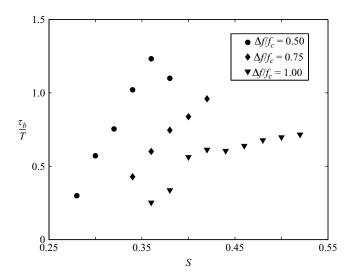
FIGURE 10. Normalized duration of single breaking  $(\tau_b/T)$  versus input slope as measured from the hydrophone. Each data point is a mean taken for single breaking events over all  $f_c$  and  $x_b k_c$  for a given value of  $\Delta f/f_c$ .
